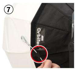
Safety attachment: Always secure the DOME and the SNAPBAG with a suitable safety cable when the primary mounting method fails, as shown in picture 6 and 7.
