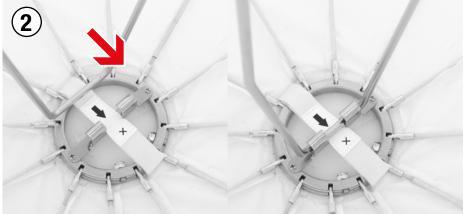
DOME instructions: Put the DOME on an even surface and push it down as shown in picture 1. By pushing the DOME down, the internal steel-stirrup approaches the two metal hooks as shown in picture 2. Make sure the steel-stirrup slides into the two hooks. In order to fold up the DOME, please push it down again and slide the steel-stirrup out of the two metal hooks.
