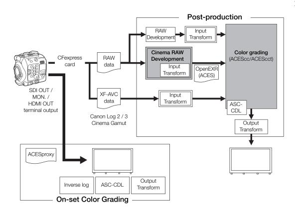
ACESproxy: ACESproxy video data that is output from the camera's output terminals when performing
