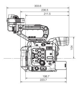
Camera with camera grip, handle unit, microphone holder, LCD monitor (open), LCD attachment unit and optional EU-V2 Expansion Unit 2
