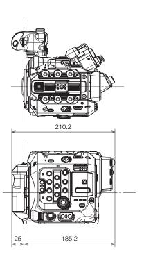
Camera with camera grip, handle unit and optional EVF-V50 OLED Electronic Viewfinder (with eye cup)
