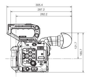
Camera with camera grip, handle unit and optional EVF-V50 OLED Electronic Viewfinder (at maximum top position)
